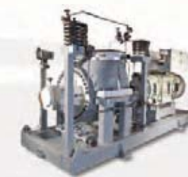
BB2 Heat transfer range Between bearings radially split range Capacity: up to 4,090m³/hr/18,000gpm Delivery head: up to 500m/1,650ft Temperature: up to 425°C/800°F Speeds: up to 3,600rpm
