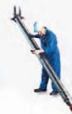
HSP Aquifer lift pump range Hydraulic submersible pump Capacity: up to 590m 3 /hr/2,600gpm/85,000bpd Delivery head: up to 1,500m/4,900ft Temperature: up to 220°C/425°F (as standard – higher temps available) Speeds: up to 10,000rpm
