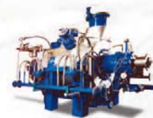
Boiler feed FK range Barrel type multistage pump Capacity: up to 2,500m 3 /hr/11,000gpm Delivery head: up to 5,000m/16,400ft Temperature: up to 250°C/480°F Speeds: 2 pole as standard & up to 7,000rpm
