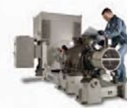
BB5 water injection range Barrel type multistage pump Capacity: up to 2,800m 3 /hr/22,000gpm Delivery head: up to 300m/1,000ft Temperature: up to 180°C/350°F Speeds: up to 7,000rpm
